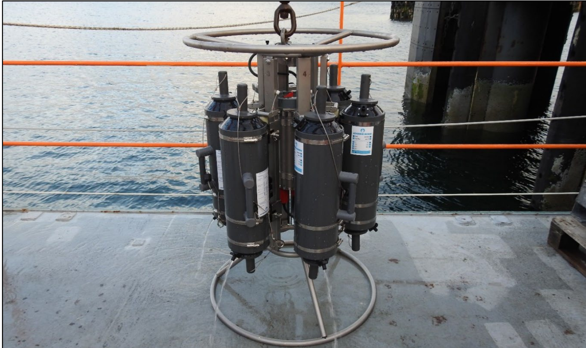
Figure 9 Rosette sampler equipped with Niskin bottles, CTD and turbidity sensor.
