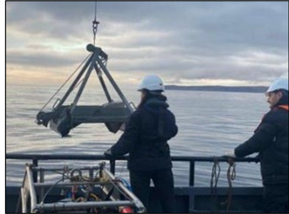
Figure 13 Hamon grab wet test (Image Source: Survey Operational Report –, 02.22.16.OPS).
